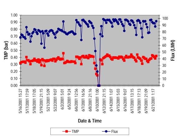
HYDRAcap TMP & Flux vs Time
