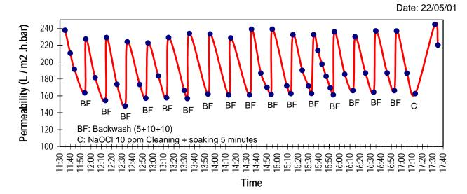
Figure 4: Backwash sequence during pilot test
